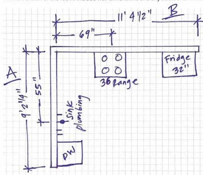
The sketch shows a kitchen layout on graph paper. Wall A is 9' 2 1/4" long. Wall B is 11' 4 1/2" long. A 36" range is positioned against Wall B, with a 32" fridge to its right. A sink base cabinet is located against Wall A, with plumbing indicated. A dishwasher (DW) is also shown against Wall A. Dimensions for Wall A are 9' 2 1/4" and 55". A dimension of 69" is shown for a section of Wall B. A dimension of 11' 4 1/2" is shown for the total length of Wall B.
